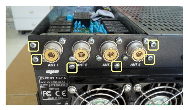
4. Then unscrew all the six fixing screws blocking the ATU module on the rear panel of the linear amplifier.
