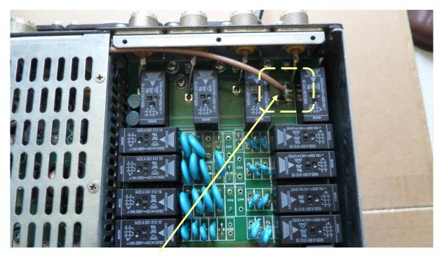
2. Then de-solder the shielded-cable shown in the picture above, being very careful with not damaging with the soldering-iron the two relays placed at both sides of the shielded-cable termination.
