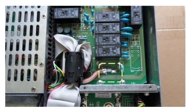
3. Repeat a similar de-soldering operation on the other shielded-cable connected at the lower side of the ATU printer circuit board, having care of making a clean operation without any relay damage.
