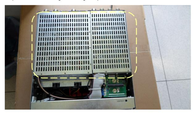
1. After having removed the top cover of the 1K-FA, take both the Power Amplifier and the ATU protection grids off in order to gain access to the underlying ATU printed circuit board. This operation can be easily performed by unscrewing all their fixing screws.
