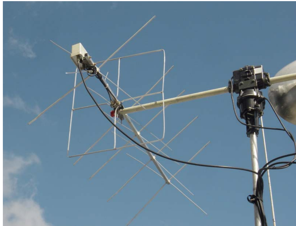
Fig 3. Isolated inputs of the new quad element
