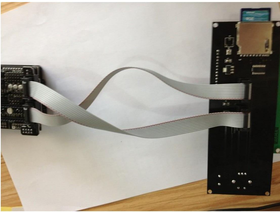
2. Add 12V power supply to the green port according to the label on the board
