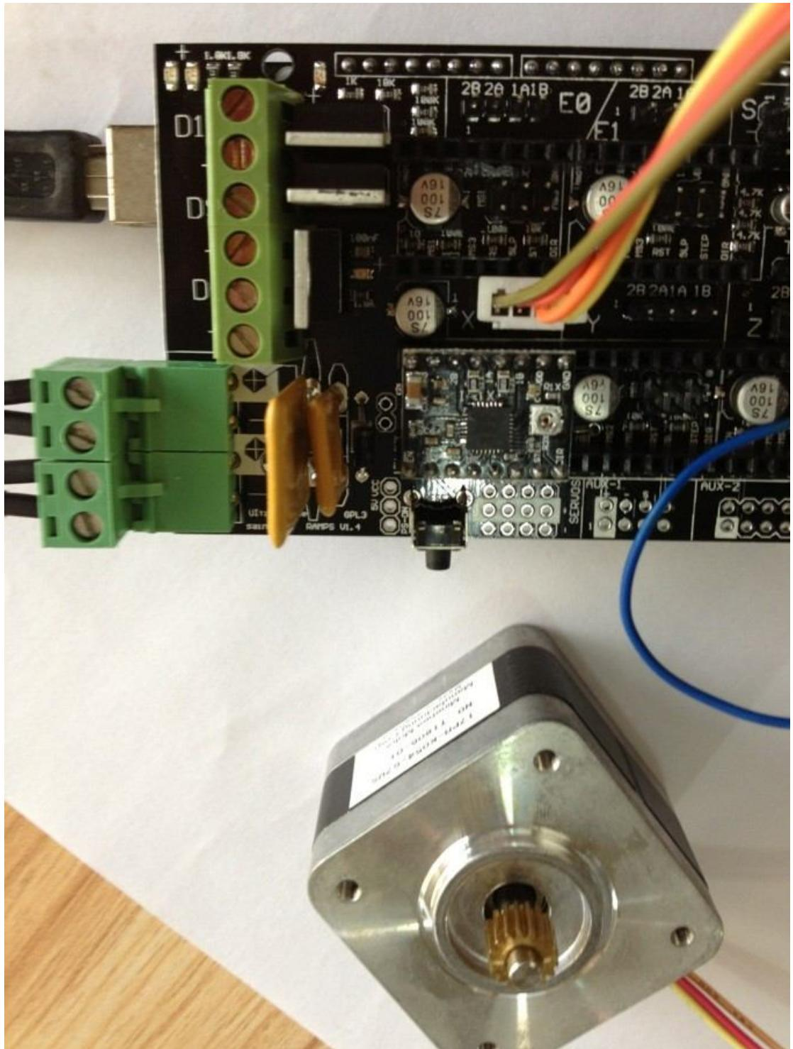
Connect 5 motors to the corresponding port on the board.
