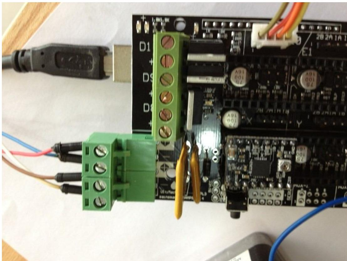
3. Wire up 2 Phase and 4 line motor. 1a 1b is 1 phase, 2a 2b is another phase. Connect the board according to the motor pins. Be careful that if it's wrong wired up, it will damage your motor. See the picture:
