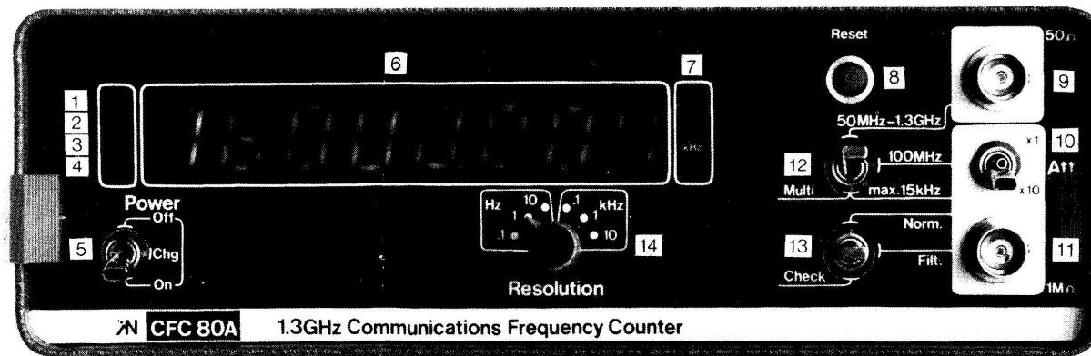
mHz (0.001 Hz) resolution is obtained. The resolution multiplier system is advantageous for measurements in the presence of noise, in that it provides reliable frequency measurements.
